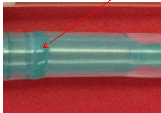
Samples of tubular " Clear-to-Pigmented " and " Natural-to-Natural " assemblies welded with laser
