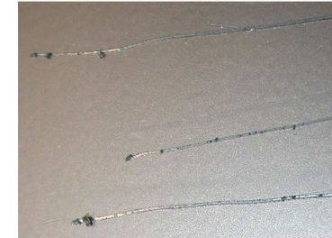
Figure 3 – Cracks in paint film extending to the substrate (due to paint softening)
