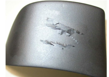
Figure 4 – Cracks in, and scratches through, the paint coating
